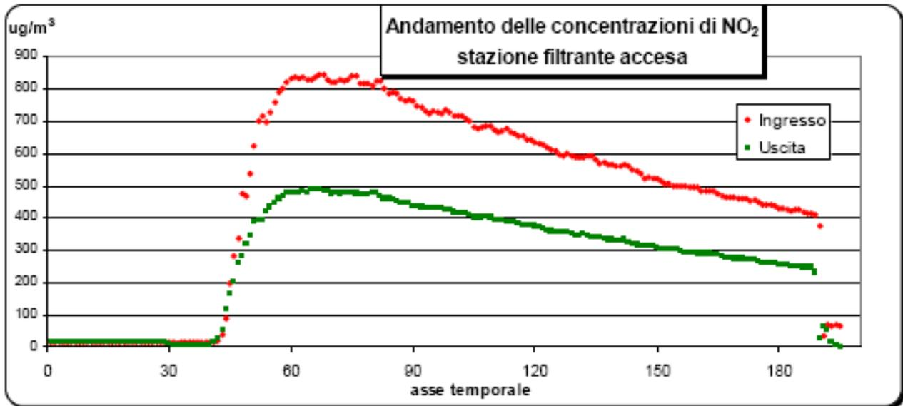
Figure 4: evolution of the concentrations measured by 2 instruments with the filtering station switched on
