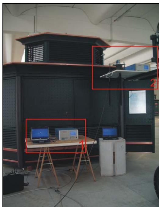
Fig.2: analysers positioned at the inlet (1) and outlet (2) mouths
