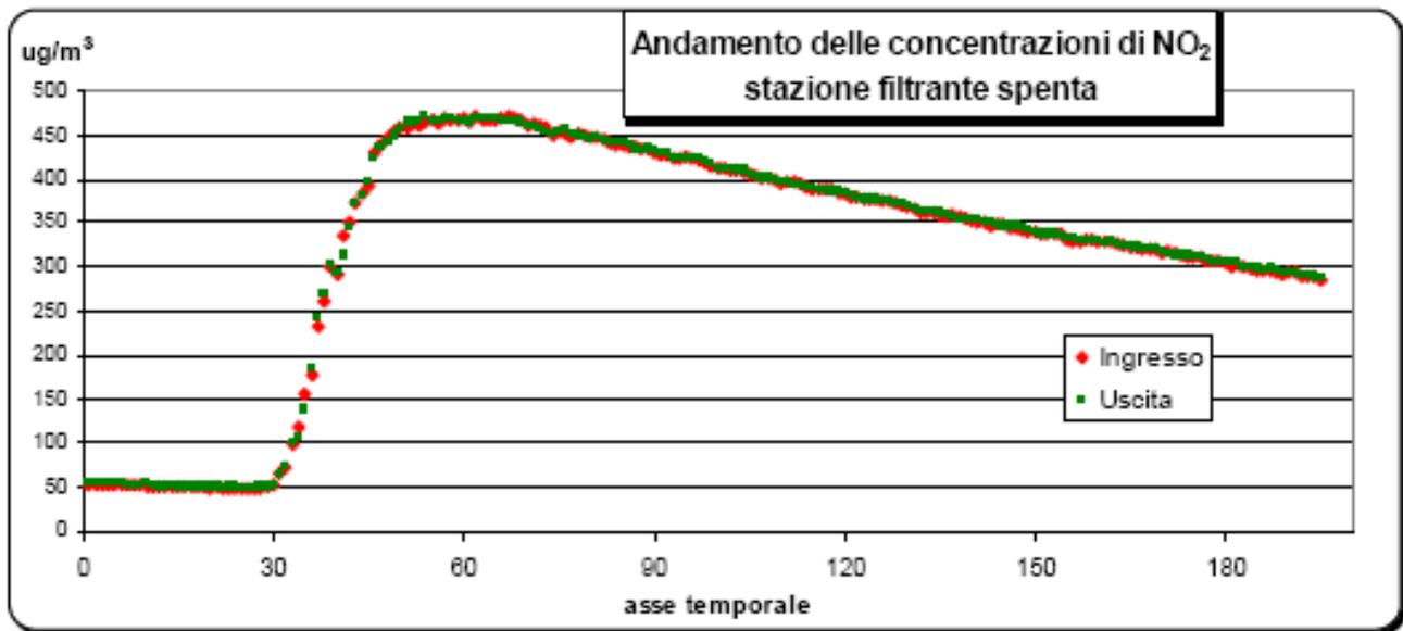
Fig. 3: evolution of the concentrations measured by 2 instruments with the filtering station switched off
