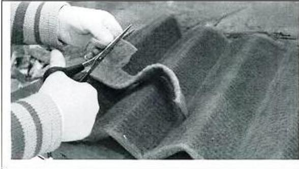
Figure 1. Cutting the "Used filter material" sample.
